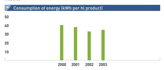
The graph shows consumption of energy per hl product. The primary reason for the decline in consumption from 2001 to 2002 is that production of carbonated soft drinks, which is less energy-intensive than beer production, increased in 2002. In 2003, beer production accounted for around 74 % of total production volume.
