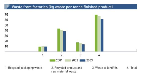
Orkla Brands focuses on reducing the amount of waste and residuals generated by its factories. The graph shows the amount of waste per unit finished product, broken down into the categories "recycled packaging waste", "recycled product and raw material waste" and "landfill waste". In the period 2001–2003, recycled packaging waste was reduced by 12 % and landfill waste was reduced by 22 %. This work will continue unabated in 2004.
