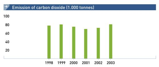
Carbon dioxide emissions from the incineration of fossil fuels at Orkla Foods remained more or less constant in the period 1998-2003, despite an increase in production of around 15 %. This is primarily due to the transition from oil and coal to natural gas and propane at several factories.
