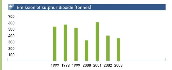
The graph shows sulphur dioxide emissions from fuel incineration at the Borregaard factories in Sarpsborg. The varying emission levels in the period 1997-2003 are due in part to the increased use of electricity rather than oil to produce thermal energy in 2000 and 2002. The transition to the use of oil with a slightly lower sulphur content and lower thermal energy requirements in the past few years have also had a positive impact on sulphur dioxide emissions.
