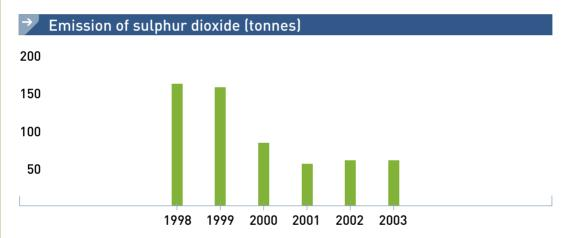
Sulphur dioxide emissions from the incineration of fossil fuels were reduced by around 63 % in the period 1998–2003 despite an increase of around 7 % in the use of thermal energy. The most important reason for this reduction was the factories' transition from oil and coal to natural gas and propane. The transition from the use of coal to the use of natural gas at the factory in Kotlin, Poland contributed significantly to this improvement.
